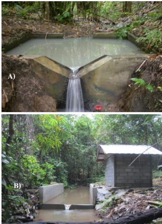
Figure 2 Streamflow measurement using water level recording and 120 ° V notch weir (A) at outlet of mixed deciduous forested watershed and at outlet of secondary forested watershed (B).
